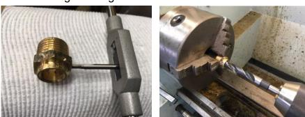
Then next step is to tap the centre of the fitting with a five eights inch and twenty four threads per inch thread tap tool. Again, this can be done by hand if need be.
