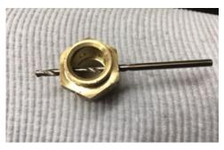
The next step was to tap the drill holes M3, then Richard put the fitting in the lathe and drilled it to nine sixteenths of an inch. This drilling can also be
