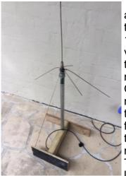
The picture on the left is of the finished antenna after tuning to be resonant in the two metre Amateur radio band of 144 megahertz to 148 megahertz. The voltage standing wave ratio was less
