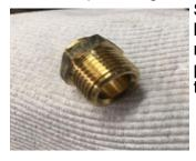
He drilled the BSP fitting on all six faces to allow later installation of the antenna radials, but he took a short cut and drilled right through
