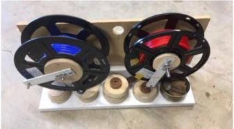
modate spool hubs with diameters between 32mm and 75mm as each supplier has different
