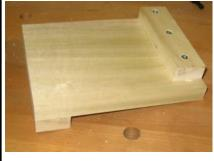
A **bench hook** minimizes the need for a vice or clamps and allows you to make quick cuts while protecting the worktop. You can use this on any surface with a square edge or even a stair tread if you don't have a work bench.
