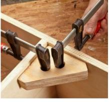
This handy little fixture is self-explanatory in layout and uses any timber offcuts with square ends.
