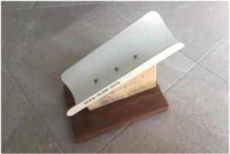
Materials needed include a piece of ninety millimetre uPVC pipe cut in half, some odd bits of wood together with some screws and some glue to hold it together.
