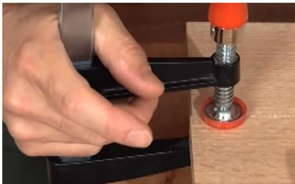
Place your boards loosely on a pair of T-bar or pipe board clamps and check the end alignment is correct. Then **one-by-one**, turn each board up in turn, run a continuous bead of glue along the length of the edge and spread evenly. How much glue to use? The answer is '**enough**'. Tighten the clamps evenly until you see **small beads of glue along the joint line**. If the edges tend to slide up, use a small F-clamp at each end to hold the boards in alignment.
