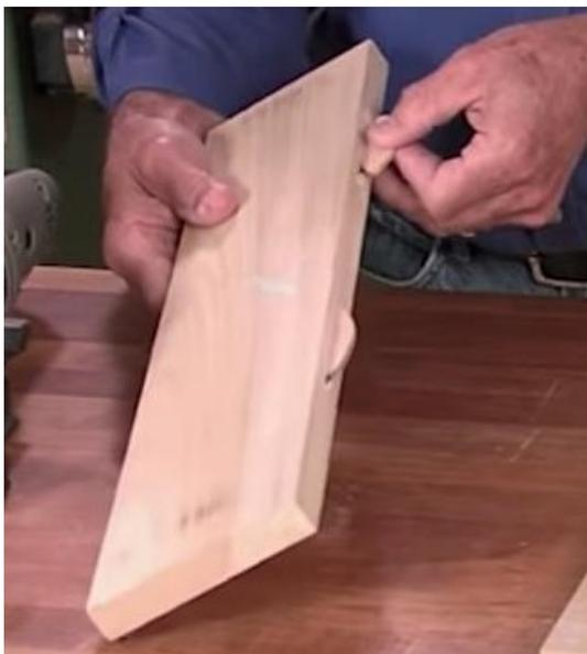
**Biscuiting (left)** is done with a special tool that cuts a **half moon slot** in the edge of the timber. **Hardwood biscuits** are coated with glue and inserted in the slots at approximately 100 to 150mm spacing.
