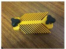
For this purpose we have various items, Shed made and/or purchased that are made from wood and plastic that are inexpensive and sufficiently soft so that they are expendable and soft enough not to cause damage to the spinning blade or cutting bit should they come into contact. It is better to mangle the bit of sacrificial wood or plastic rather than your finger.
