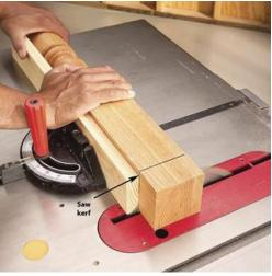
measure, or speed up multiple identical cuts by using a pattern stick or stop block.) If you want even more precision, here's a great tip to allow you to see exactly how much of the stock board the kerf will consume. Begin by making a partial cut into a scrap piece of lumber. This will leave a shallow channel in the surface of the material that you can measure to make
