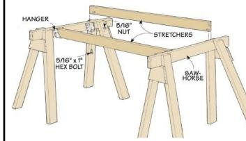
To keep the stretchers from accidentally slipping out of the hangers, they fit onto a metal pin in each hanger. This "locking" pin is just a bolt that passes through a hole drilled in the joist hanger, tightening a nut on the end of each bolt holds it in place. To fit the stretcher over the bolt and nut, all you need to do is drill a pair of counter bores near the end of each stretcher.
