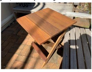
Almost a week later, Richard wrote again: "I built this foot step using my table router with all joints glued with epoxy and finished with Tung Oil. 250mm high to reach those higher shelves, made from 285w x 19t shelf pine. Next is another antenna project."
