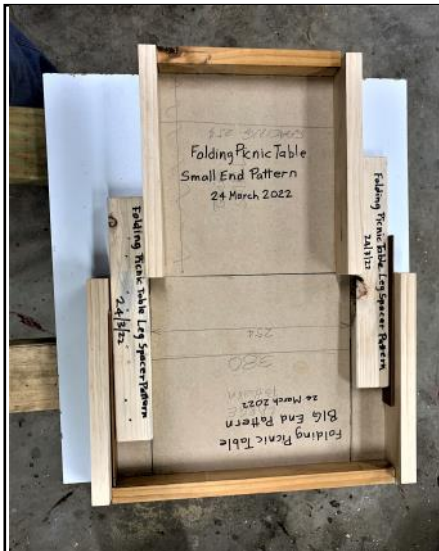
The pattern during manufacture. Clearances are critical to ensure folding
