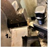
Facing the end after cutting off the original bevel
