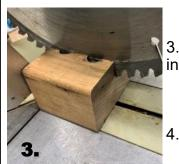
3. Cutting the work holder so it can be clamped in the mill
