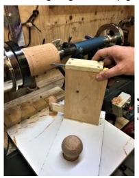
**Tom Wolf's 1:350 scale** model of *HMT Dunera* is progressing. This model is being built with the "bread and butter" method (thin layers of timber for each deck on top of each other making a solid hull) and the jig is complete, the hull itself is a work in progress (right).
