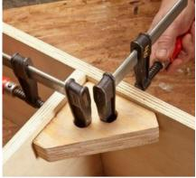
This handy little fixture is self-explanatory in layout and uses any timber offcuts with square ends.
